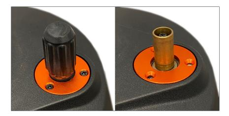
Remove the rubber focuser knob from the telescope. Sometimes they are tight but wiggling it while pulling will remove it. Remove the 3 screws from the orange plate around the focus shaft. Leave the plate in place.
