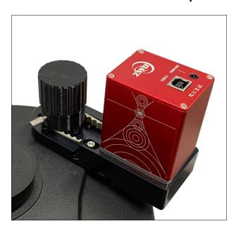
Note the slots on the bottom side of the Motor Bracket; these will line up with the raised sections of the Telescope Bracket. Place the Motor Bracket in place, close to the knob, and make sure the timing belt fit around the teeth on the Motor Pulley. Pull the Motor back away from the knob to tension the belt and use the included  $6-32 \times 5/8$ " socket head screws and 7/64 hex wrench to attach the two brackets together.
