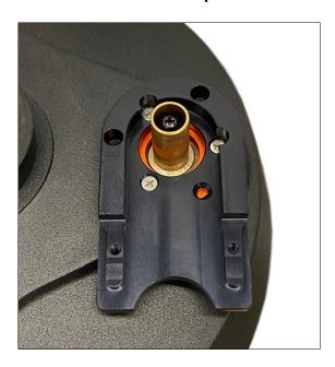
Use the included M3  $\times$  12mm flat head screws to attach the Telescope Bracket to the telescope. The inner set of 3 holes are used for 6", 8" and 9.25" scopes. Make sure the brass focus shaft stays centered through the orange plate when tightening down the screws. This will avoid binding.
